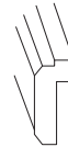
Light Rail Molding ●LRM8-SH=2 1/4"Tx96"L Shaker Style ●LRM8=2 1/4"Tx96"L Raised Panel Style
